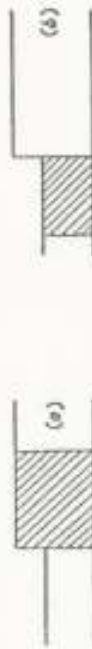
Fig. 2.8. Effect of dielectric on one side of a discontinuity. C'_d is multiplied by \kappa_r in (a) but not in (b).
