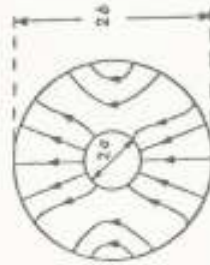
Fig. 2.4. Electric field pattern in a coaxial line for the next mode above the principal.
